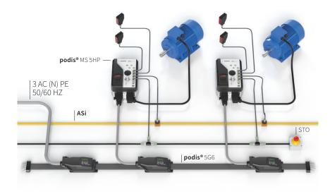
Decrease material and reduce costs with the podis® power bus system. Make planning more flexible and distribute power to the motor at any position. Connect wires with insulation displacement technology.
